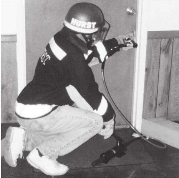
To operate quick disconnect couplings, push the quick disconnect connectors from pump and hose together. Rotate the coupling sleeve 1/4 to 1/2 turn to lock the connection.
